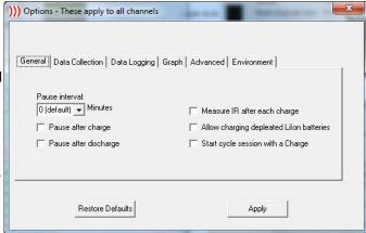
If you have checked the option to 'Measure IR after each charge' then the IR test will occur following the pause. This allows the battery to cool and stabilize prior to measuring the internal resistance and starting a new discharge cycle if applicable.
