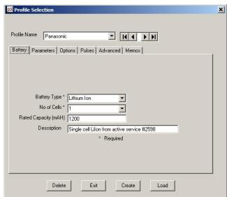
No of Cells: This is the number of cells connected in series. This is a required field.
