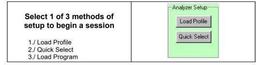
When using the *Load Profile* or *Quick Select* method the user does not need to concern themselves with selecting the correct charging algorithm for constant current or constant voltage. BA500WIN will automatically select this for you once you select the battery type.
