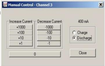
The charge and discharge currents are all constant current, fully regulated by the analyzer. You have the ability to specify and adjust the current in 1mA increments. There is no voltage regulation during charge. So be careful if using this to put charge current into a SLA or Lilon type battery. The voltage can rise up and damage the battery. Also there is no voltage cut-off during discharge so the battery voltage can go down to 0 and damage the battery.
