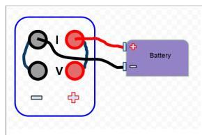
Analyzer being used with a **2 wire battery connection**. Note the jumpers connecting each pair of terminals at the analyzer.
