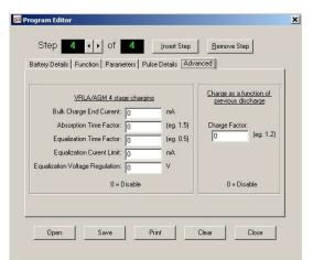
The Advanced tab has inputs for specifying Absorption and Equalization options. See the section on Profile Selection for details on how to use these Advanced features.
