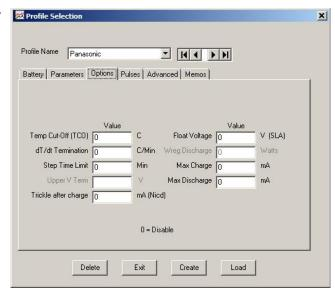
within this time then the analyzer will enter into the next step. The next step might be a pause or the start of discharge for the next cycle. Enter the value in minutes. A value of 0 will disable this feature.
