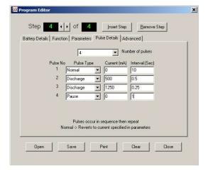
As with parameters you can also define different pulse definitions for each of the steps in the program. If you do not want pulses applied during the step then set the number of pulses to 0. This will disable all pulsing for this step and the current will be as specified in the Parameters for this step. Specify up to 6 different pulse definitions
