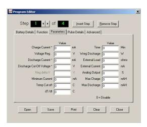
The Parameter tab is used to enter all test parameters for the presently displayed step. The explanation for each of these fields is the same as when using Profiles.
