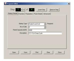
This first tab *Battery Details* is where you can enter some information about the battery under test. The *Battery Type* field will configure the correct charging algorithm required for the various battery types. The *No of Cells*, *Rated Capacity* and *Description* fields are for information purposes only and do not affect the operation of the program. This information will appear on the printed program report.
