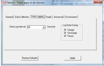
log file. This is repeated continuously until the session completes. You are not limited to the values in the drop down box. Enter any value in seconds.
